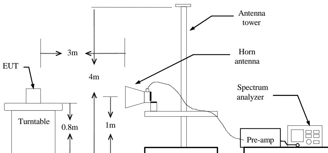
**Substituted Method Test Set-up**
