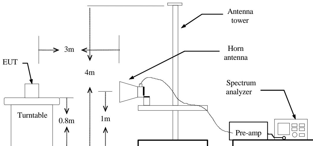
**For Substituted Method Test Set-UP**
