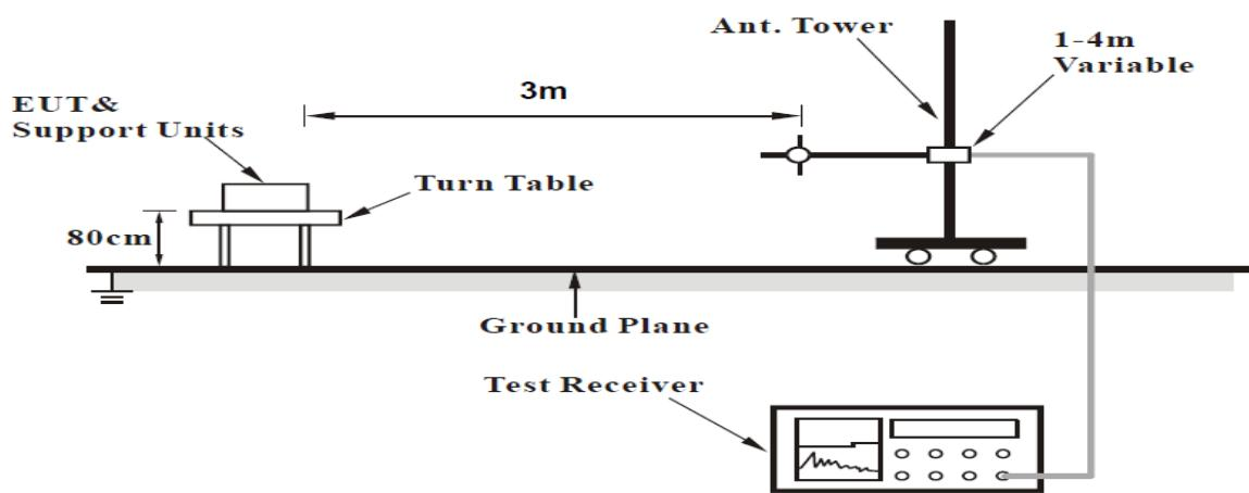
3. Radiated Emission Test Set-Up, Frequency Above 1000MHz.
