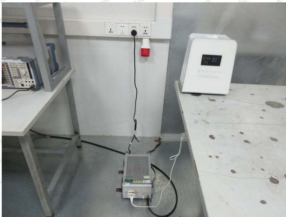
Photo of Conducted Emission Measurement
