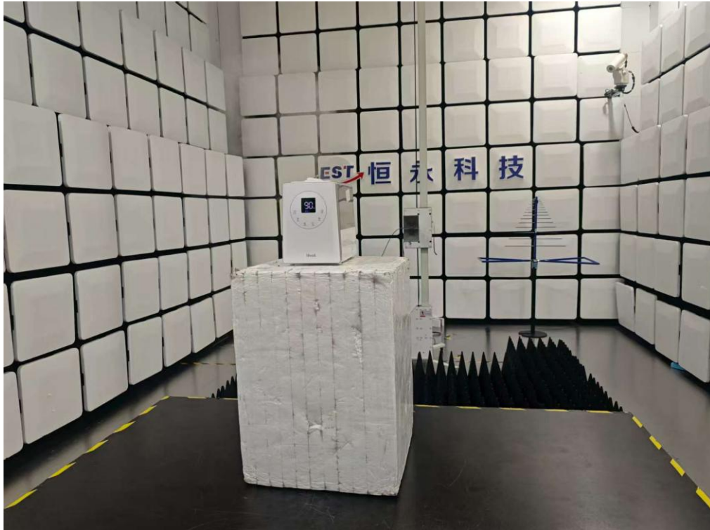
Radiated Test (Above 1GHz)
