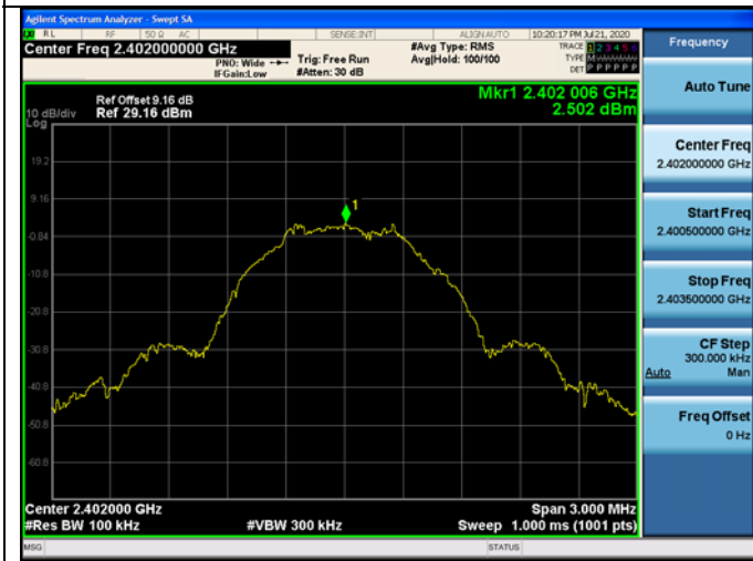
GFSK on Channel 00
