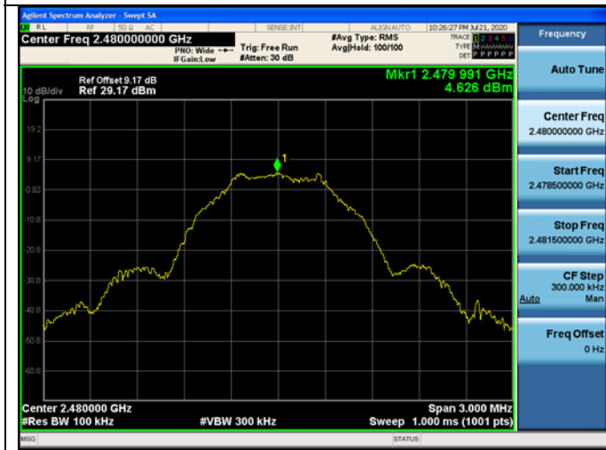
GFSK on Channel 39
