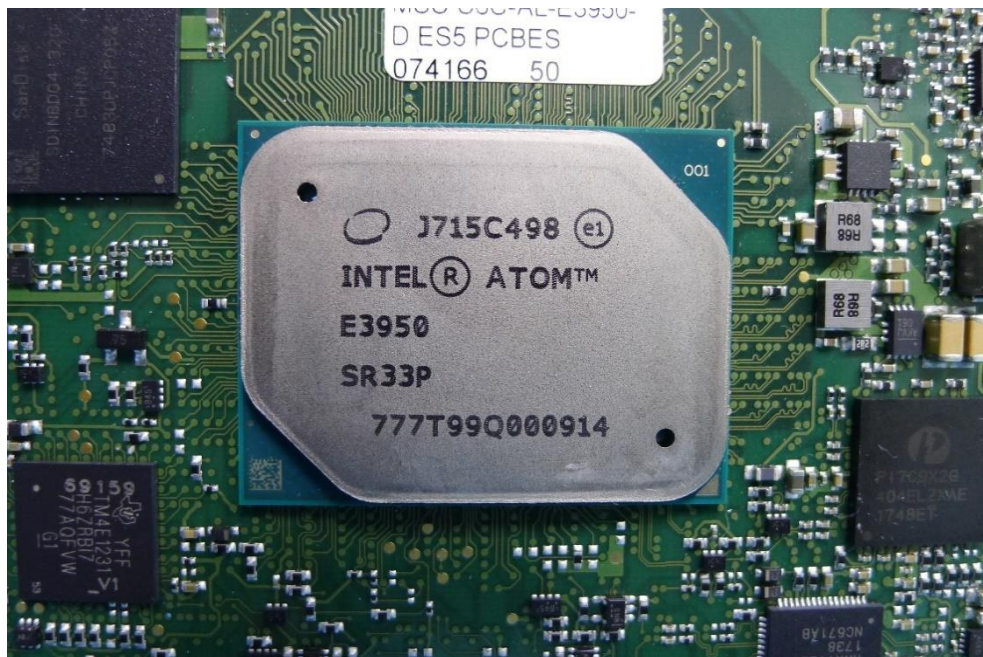
(24) CPU Board (Intel Atom E3950)
