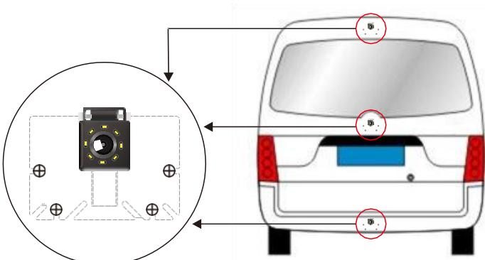
3. Route the camera video & Power cable inside the cab, and connect the AV connector and power connector to the wireless Transmitter.
