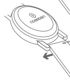
3. Push the spring bar into the other side, your new strap is installed!
