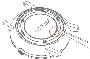
4. Install the new battery (CR2032) in the same way as removing it. Once it is properly installed, the indicator light will flash red once
