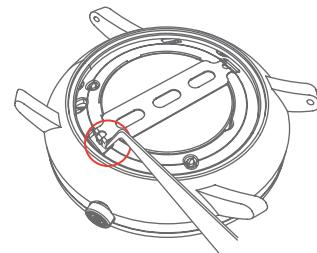
3. Take out the old battery by using tweezers or a flat tool thinner than 2mm, carefully lift and remove the battery.
