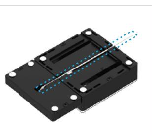
Insert the USB cable of the Camera Button Module through the Device Module centerline groove and fix it.
