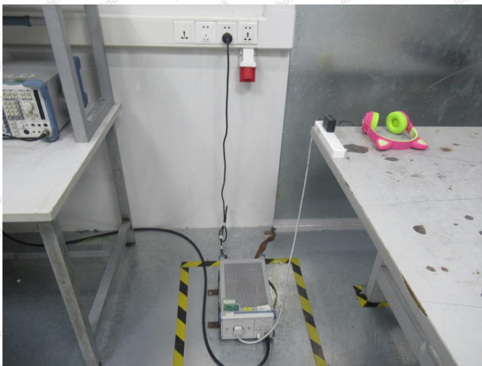
Photo of Conducted Emission Measurement
