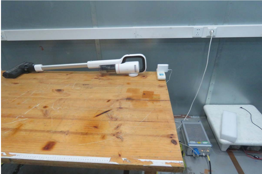
Picture 2 Conducted Emission Test Setup
