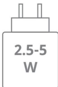
The power delivered by the charger must be between min 2.5 Watts required by the radio equipment, and max 5 Watts in order to achieve the maximum charging speed.
