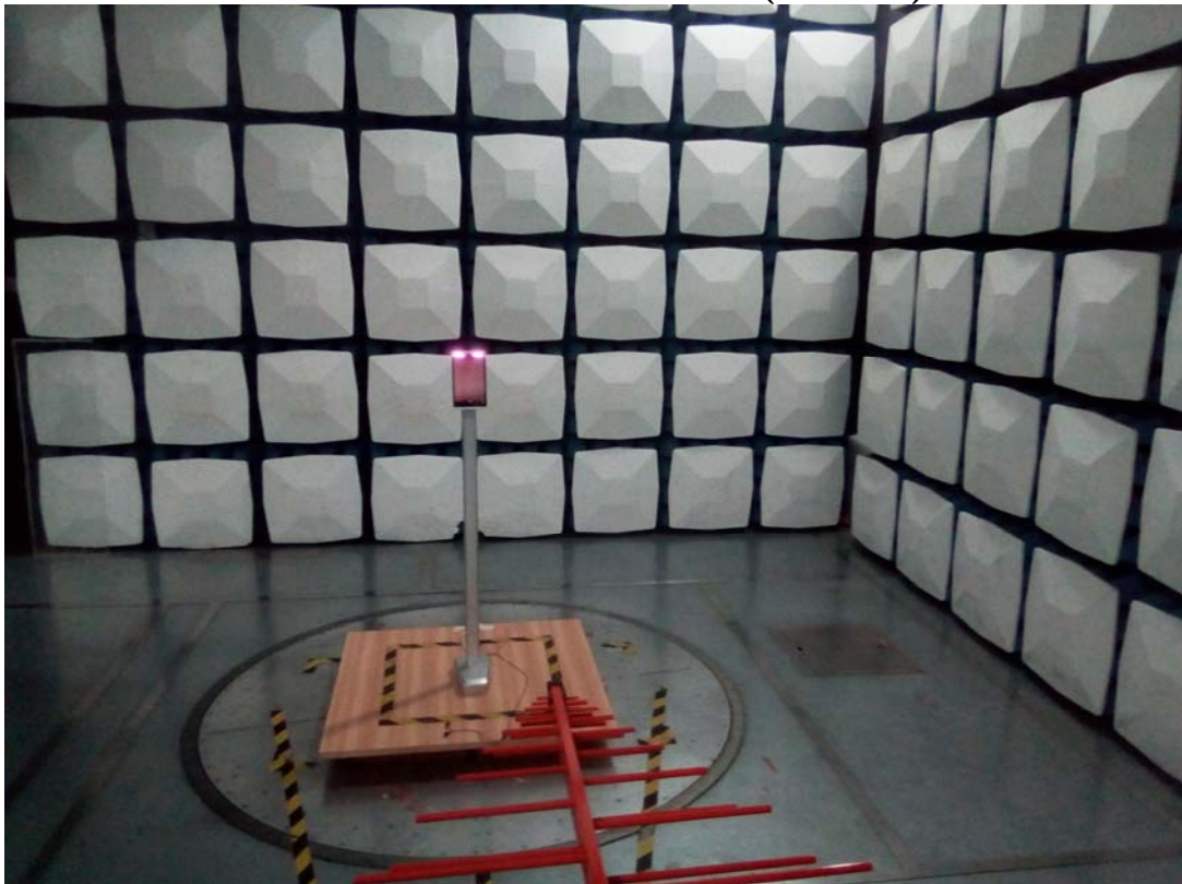
Radiated Emission Below 1GHz View(AC Power)
