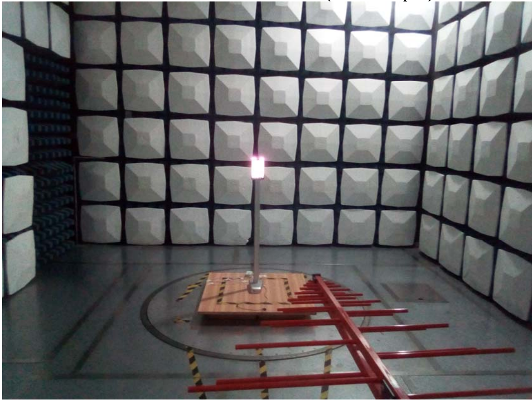
Radiated Emission Below 1GHz View(AC Power)
