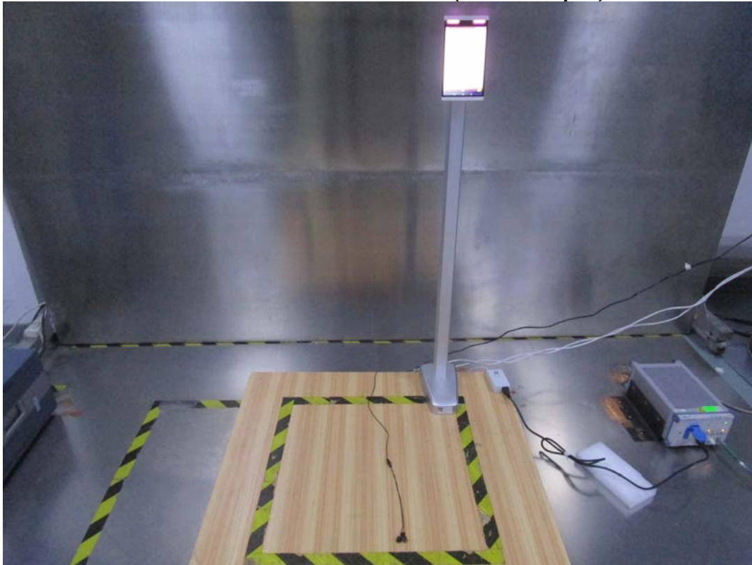
Conducted Emissions – Side View(AC/DC Adapter)
