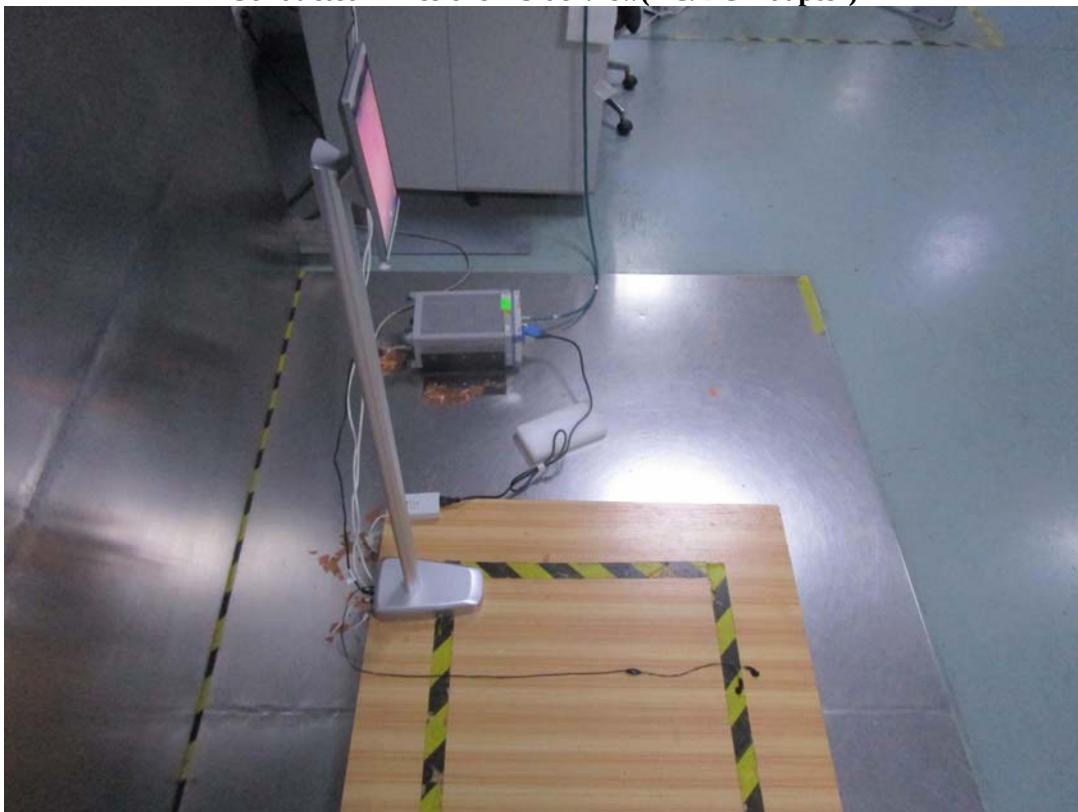
Conducted Emissions – Side View(AC/DC Adapter)
