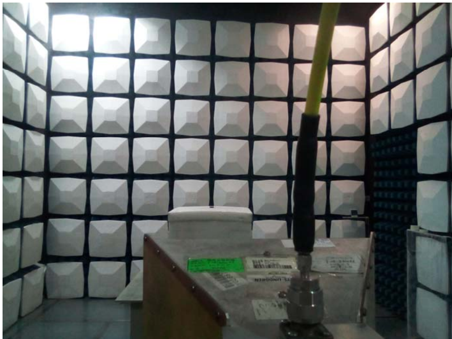
Radiated Emission Above 1GHz View
