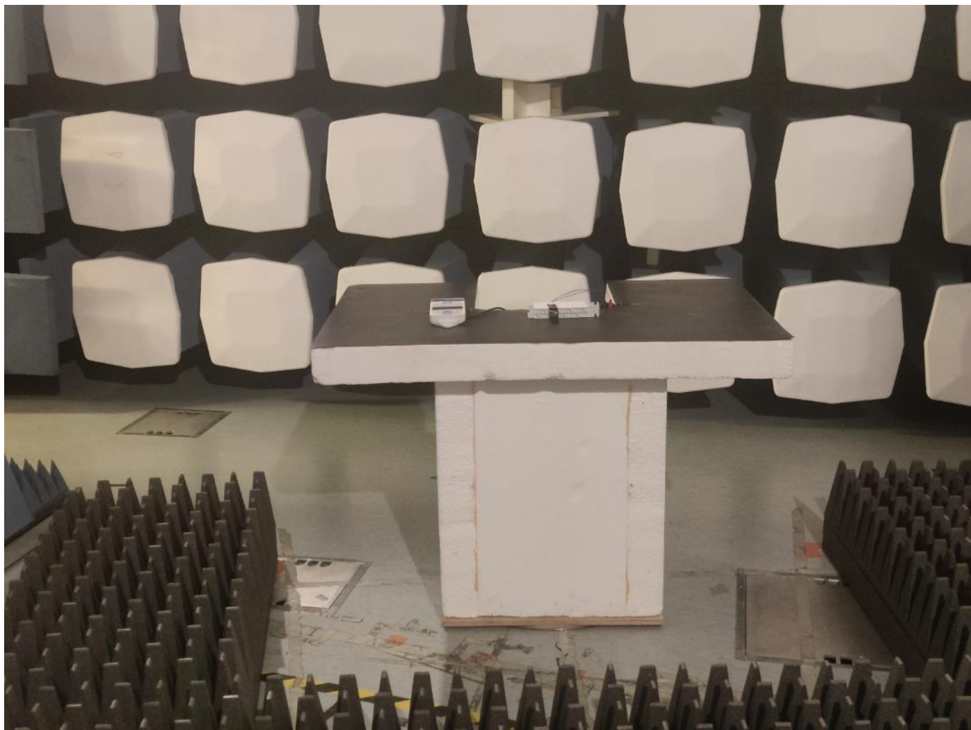
Picture 12 Radiated emissions, EUT setup 30 MHz – 18 GHz, front view
