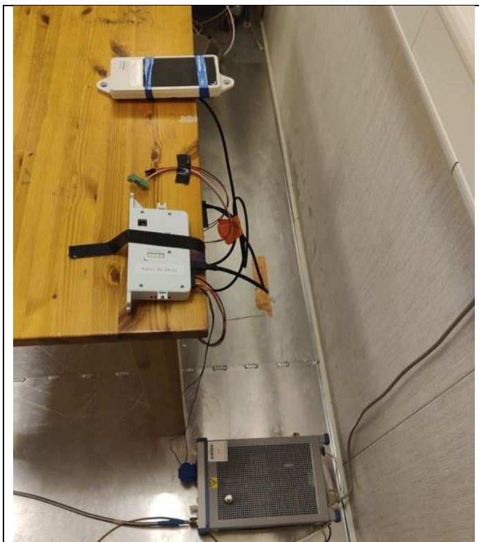
Picture 9, AC Power Line Conducted Emissions
