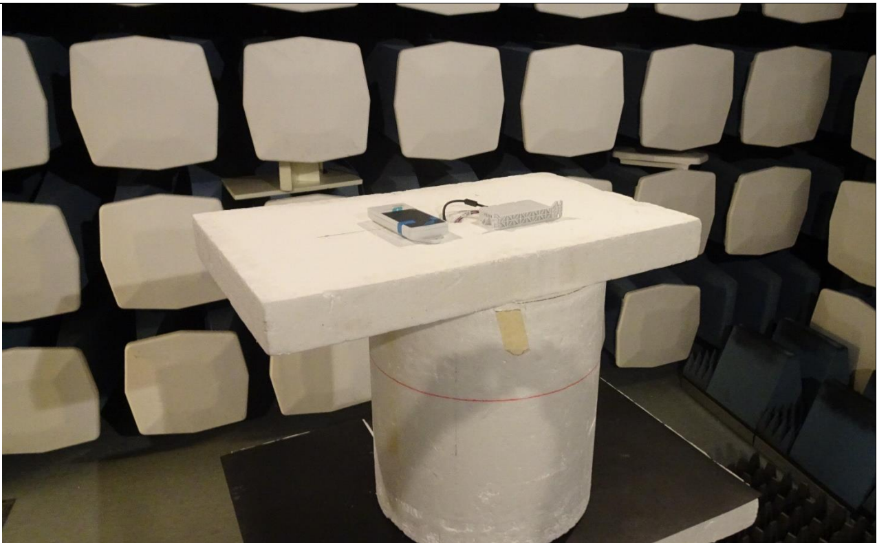
Picture 20, Radiated Spurious Emissions, EUT setup, TX 1 – 26 GHz, front
