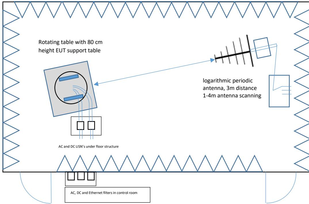
Radiated measurements setup from 1 GHz to 18 GHz:
