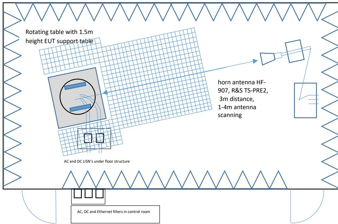
Radiated measurements setup from 18 GHz to 26 / 40 GHz:
