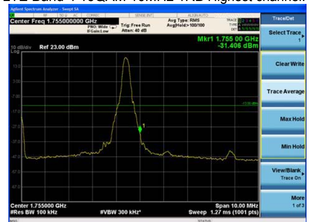
LTE Band 4 16QAM 10MHz 1RB Highest channel:
