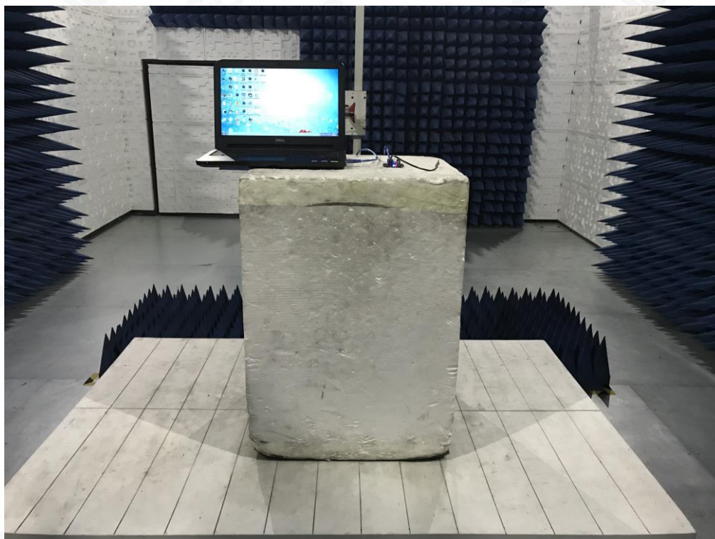
FCC RADIATED EMISSION TEST SETUP ABOVE 1GHZ
