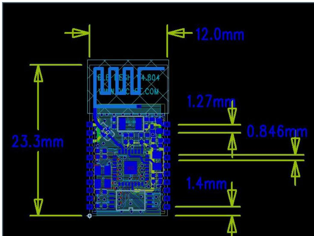
Module size is 23.3\*12 mm, pin spacing is 1.27 mm, pin foot width is 0.846mm.
