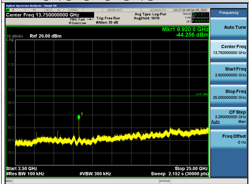
Test_Graph_EDR_ANT1_2480_2Mbps_Higher Band Emissions
