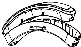
Move the toggle switch at the buckle and simultaneously pull the battery up until the battery and battery compartment are completely separated.
