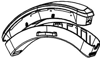
1 . Firstly, insert the hole under the charging port end into the battery compartment socket.
