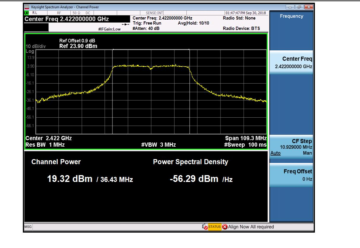
**Maximum peak conducted output power\_11N40SISO\_2442\_Ant1**
