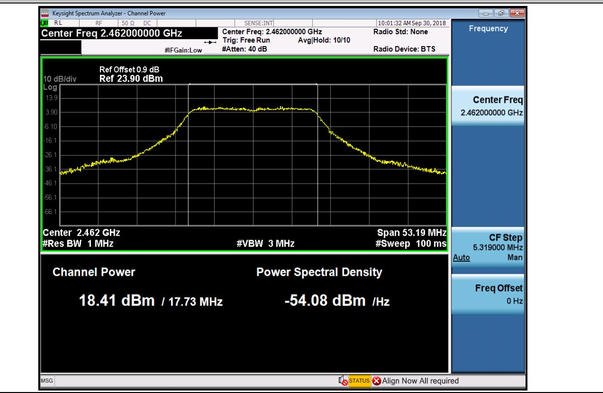
**Maximum peak conducted output power\_11N40SISO\_2422\_Ant1**
