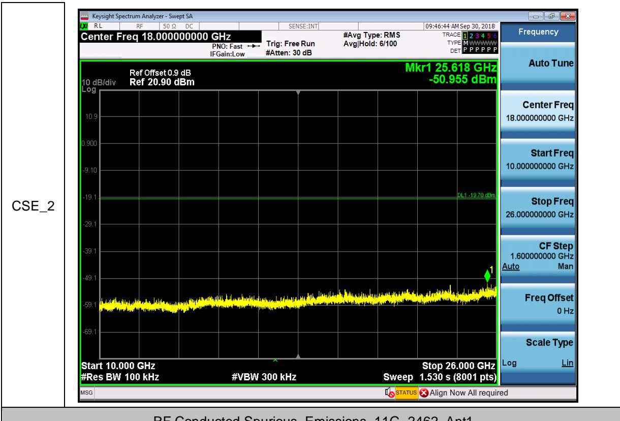
RF Conducted Spurious Emissions\_11G\_2462\_Ant1
