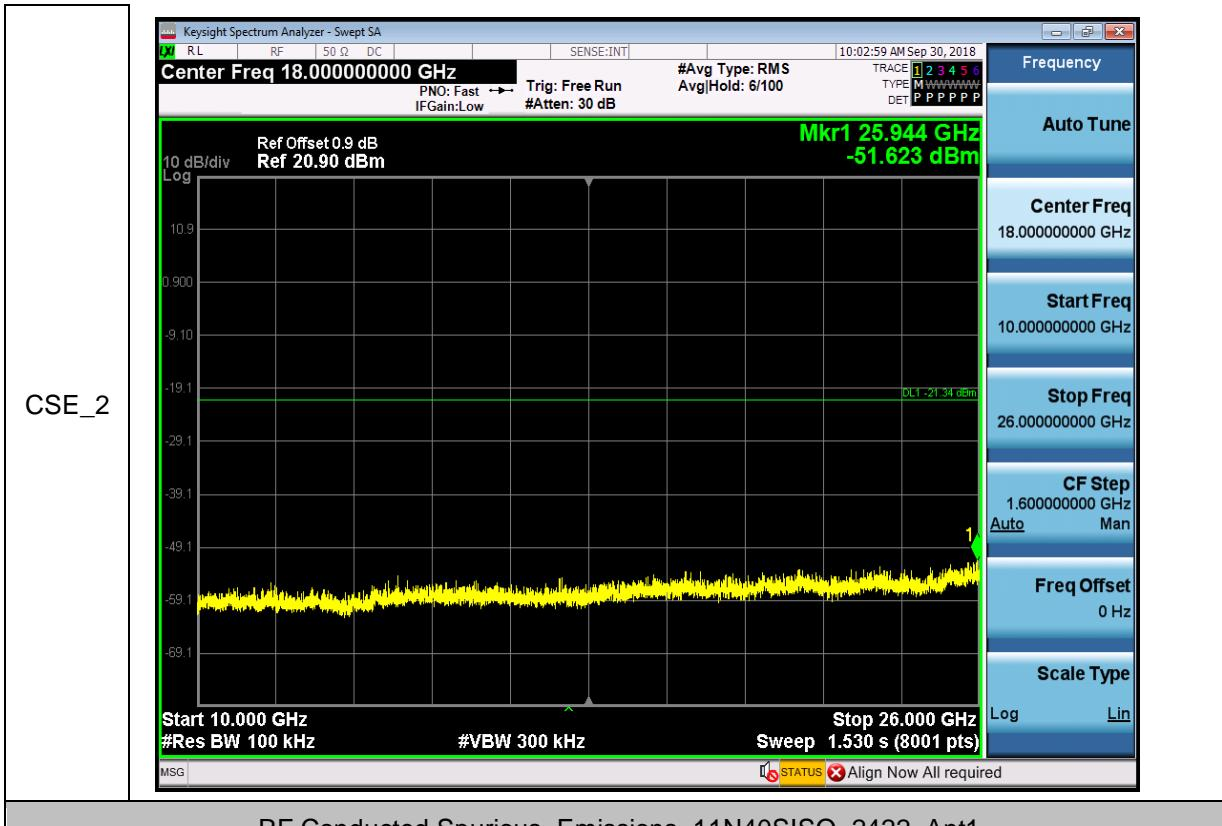
RF Conducted Spurious Emissions\_11N40SISO\_2422\_Ant1
