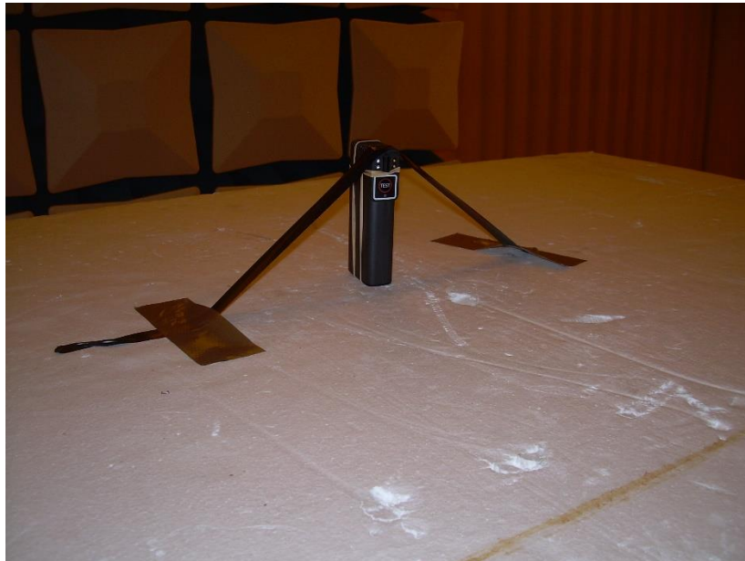
Photograph 8: Front View Radiated Emissions Configuration – Above 1000 MHz – Vertical Battery Powered
