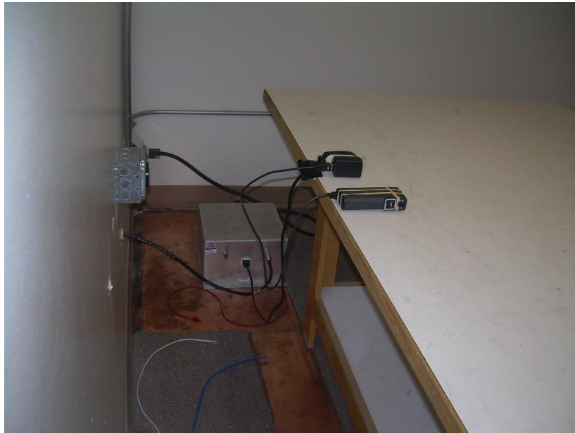
Photograph 10 – Back View Conducted Emissions Worst-Case Configuration
