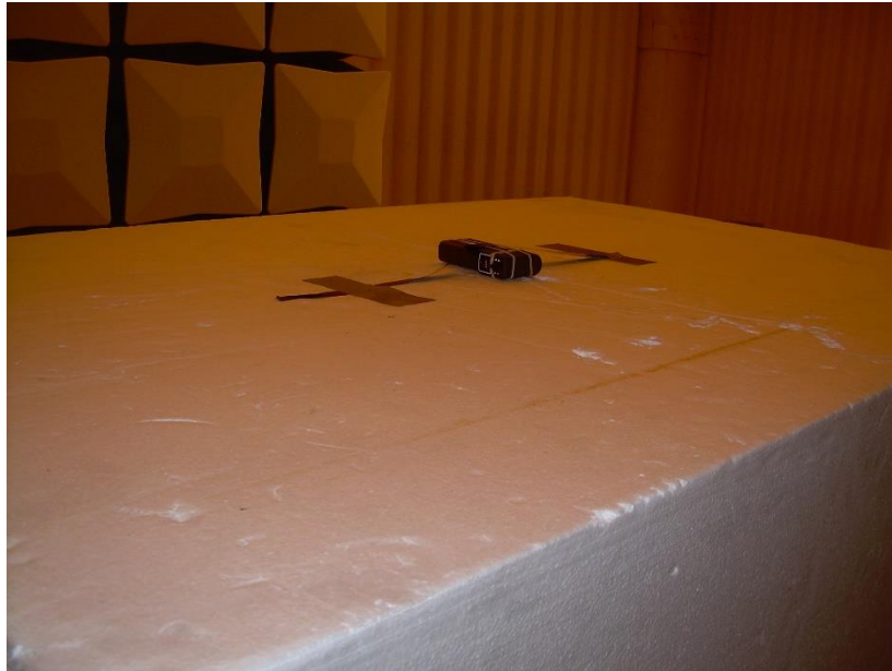
Photograph 7: Front View Radiated Emissions Configuration – Above 1000 MHz – Flat Battery Powered
