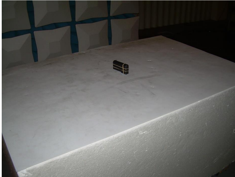
Photograph 1: Front View Radiated Emissions Worst-Case Configuration – Below 1000 MHz – On Edge Battery Powered
