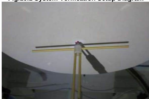
Fig.10.2 Photo of Dipole setup
