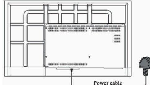
Step 2: Turn on the Rocker switch (back side of the monitor, next to power outlet). Enter standby state, the power indicator turns to red color.
