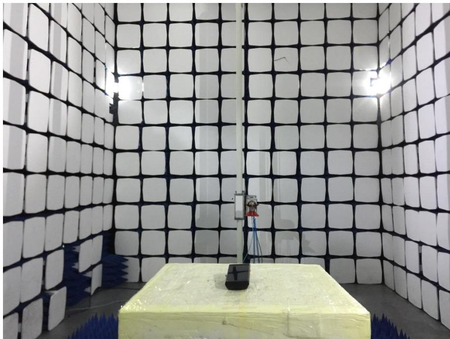
**Radiation Emission Test Setup (Above 18GHz)**
