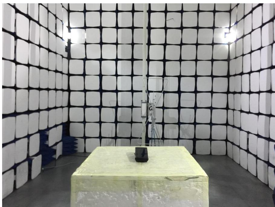
**Radiation Emission Test Setup (1GHz to 18GHz)**
