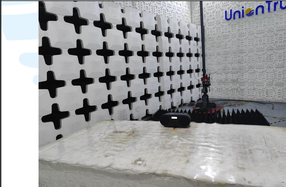
Radiated emission Test Setup-2 (Above 1 GHz)
