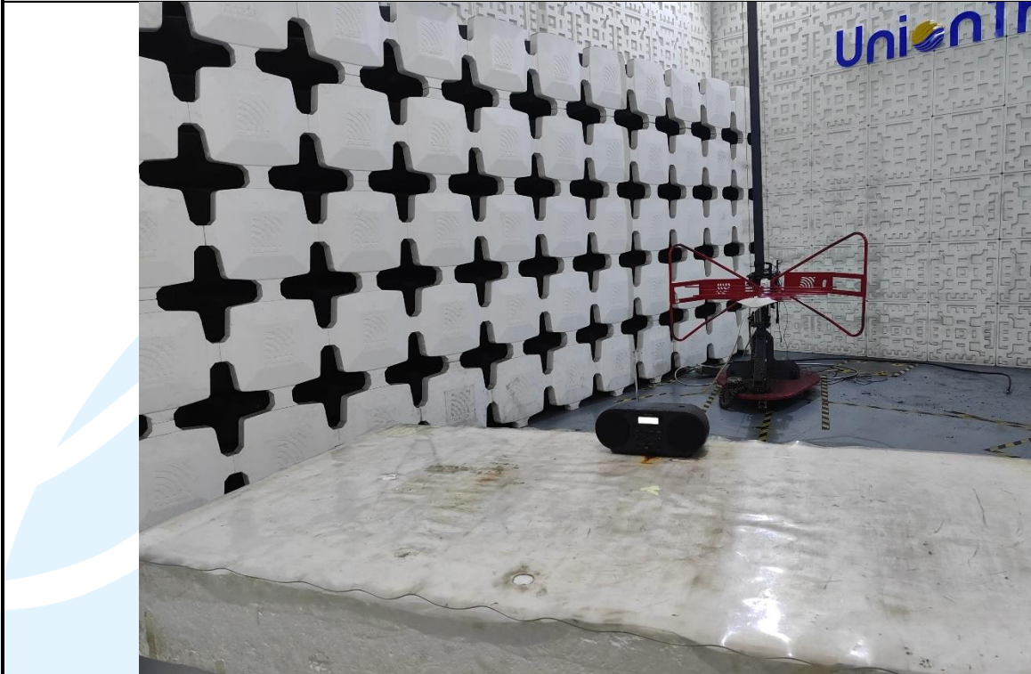
Radiated emission Test Setup-1 (30 MHz~1 GHz)
