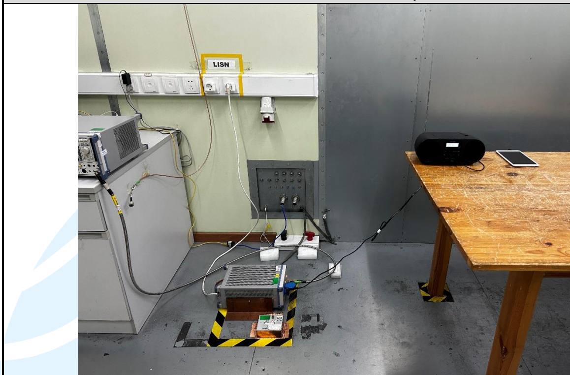
Conducted Emission Test Setup-3
