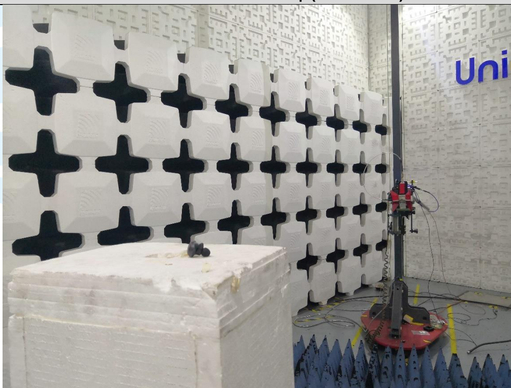
Radiated emission Test Setup (Above 1 GHz)
