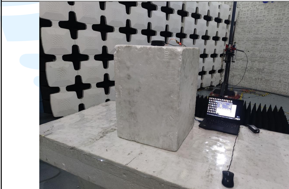
Radiated emission Test Setup (Above 1 GHz)
