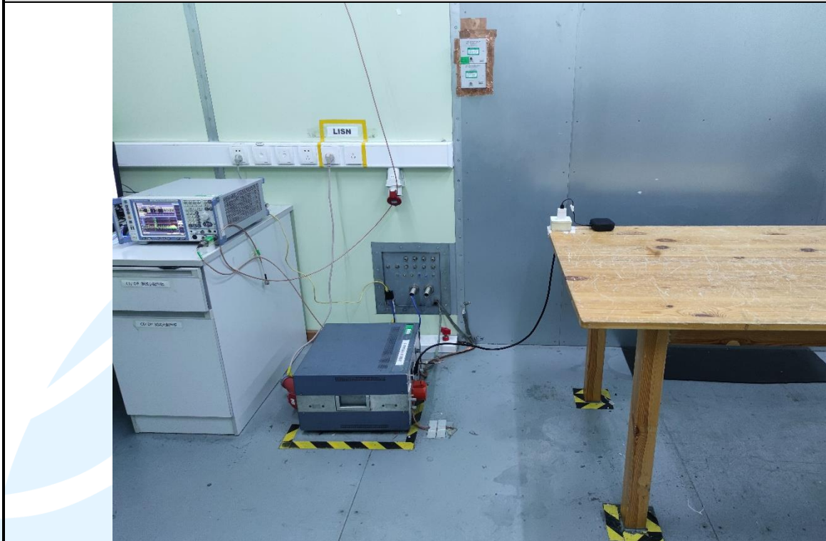
AC Power Line Conducted Emission Test Setup
