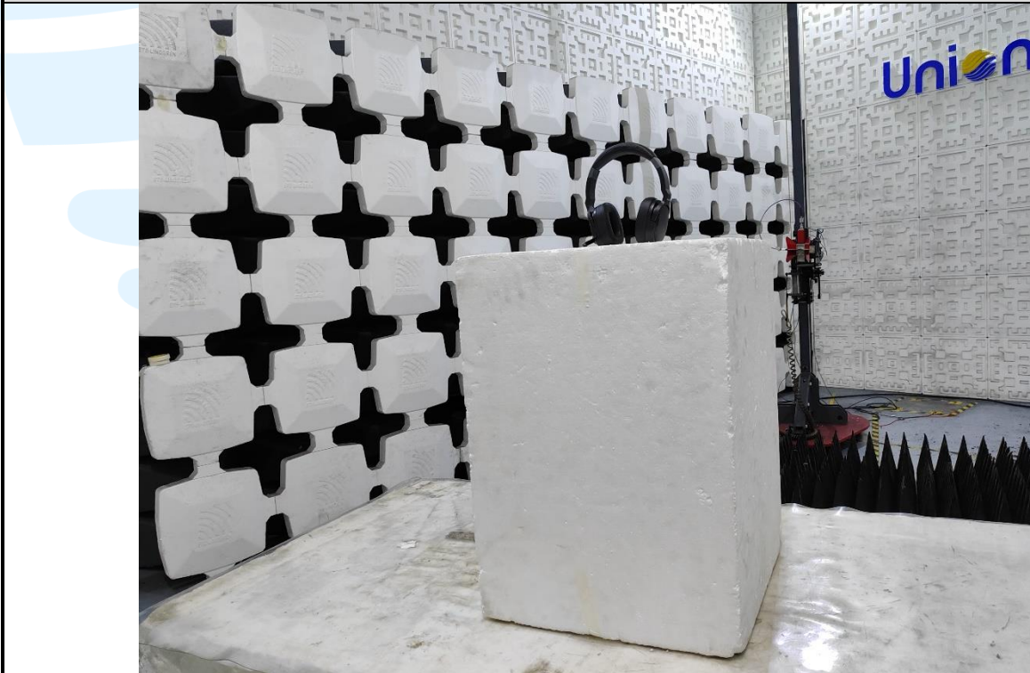
Radiated emission Test Setup (Above 1 GHz)
