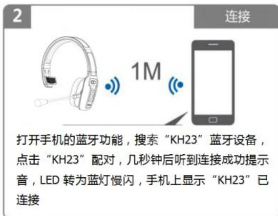
1. In off status, long press MFB for 5-7 seconds to enter pairing mode with Blue & Red LED flash alternately.
