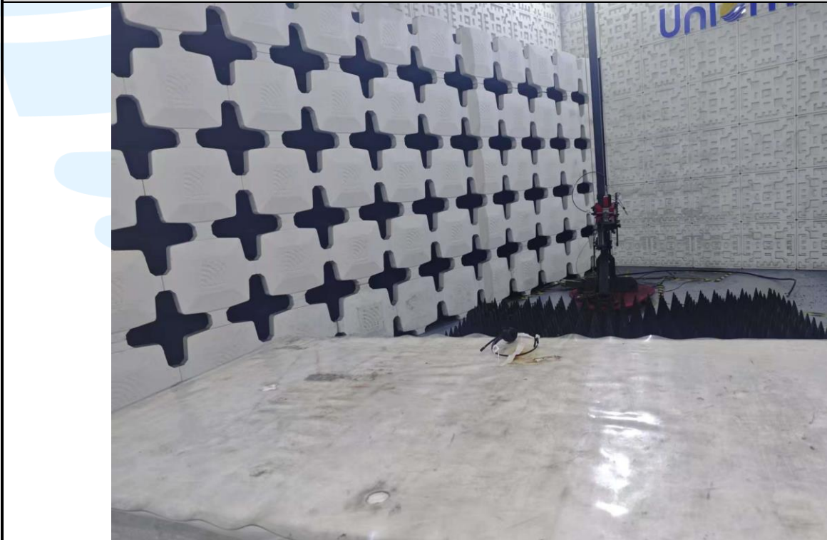
Radiated emission Test Setup-2 (Above 1 GHz)
