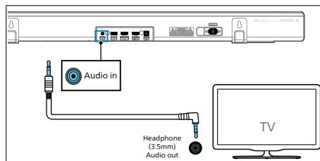
2 Use a RCA to 3.5mm audio cable to connect the TV's audio output sockets to the **Audio in** socket on the unit.
