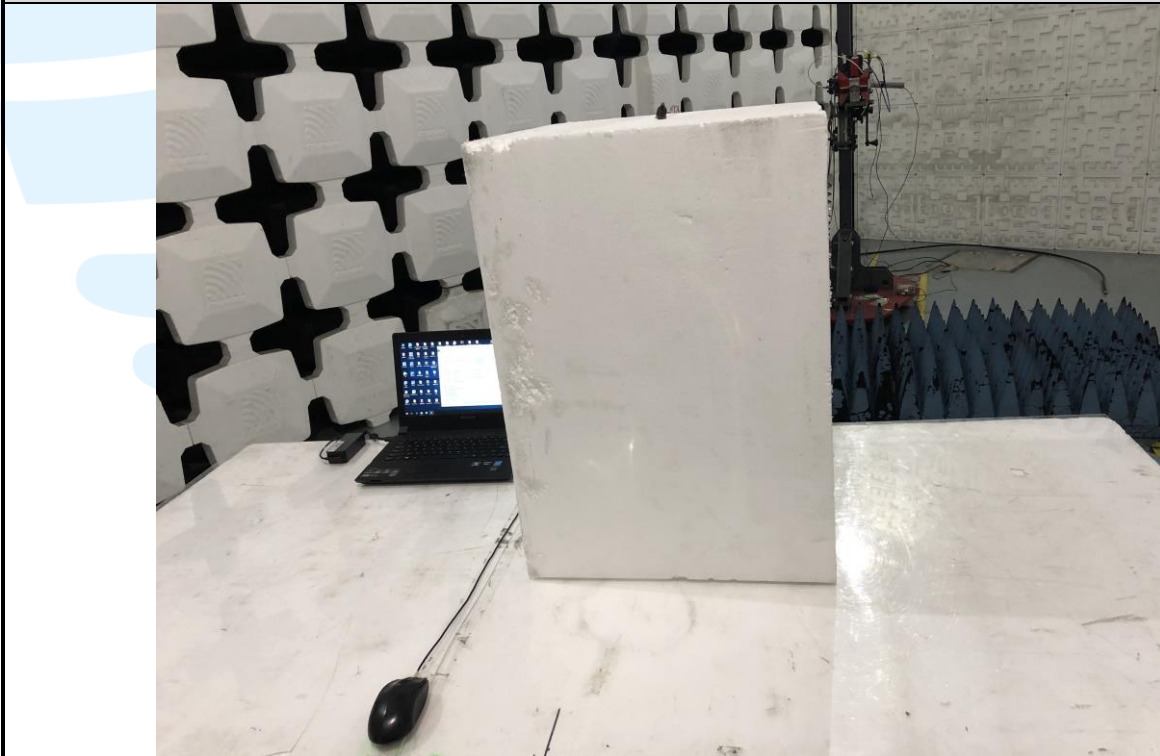
Radiated emission Test Setup (Above 1 GHz) -Right
