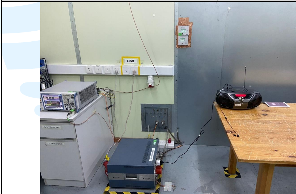
Conducted Emission Test Setup
