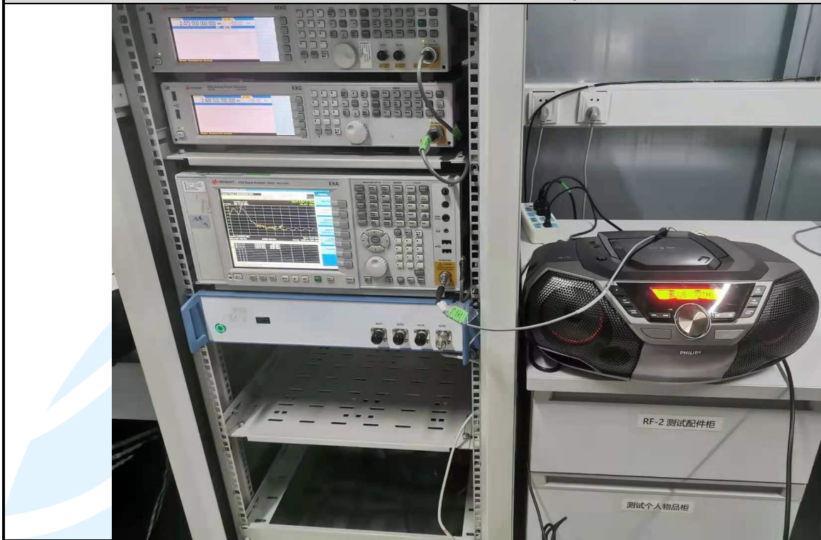
RF Conducted Test Setup
