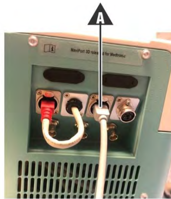
Figure: Plugging Ethernet Cable to Ziehm Monitor (A)
