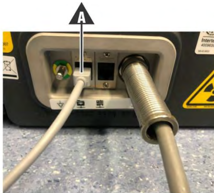
Figure: Plugging Ethernet Cable to Brainlab Airo Workstation (A)
