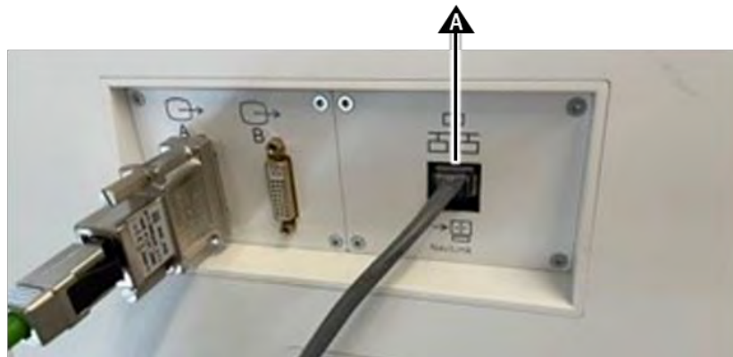
Figure: Plugging Ethernet Cable to Cios Spin Monitor (A)
