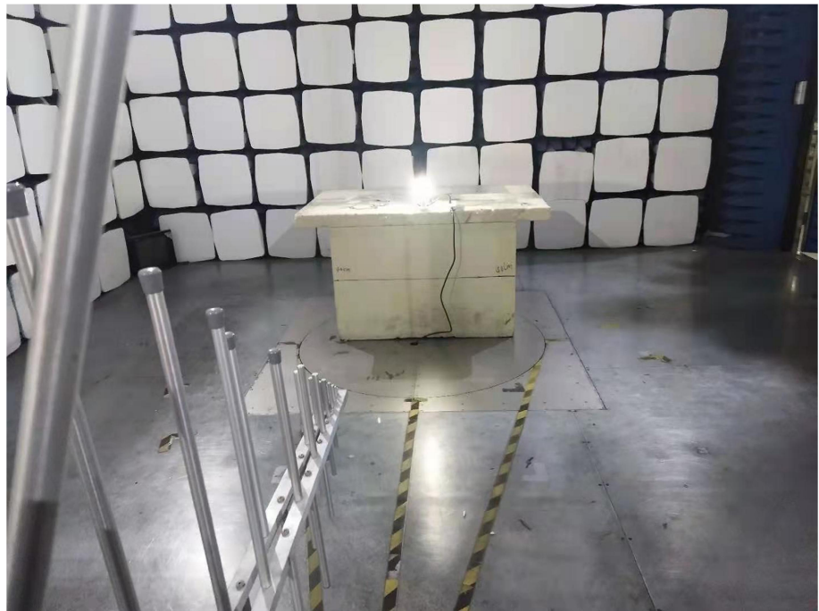
Radiation Emission Test Setup (30MHz to 1GHz)
