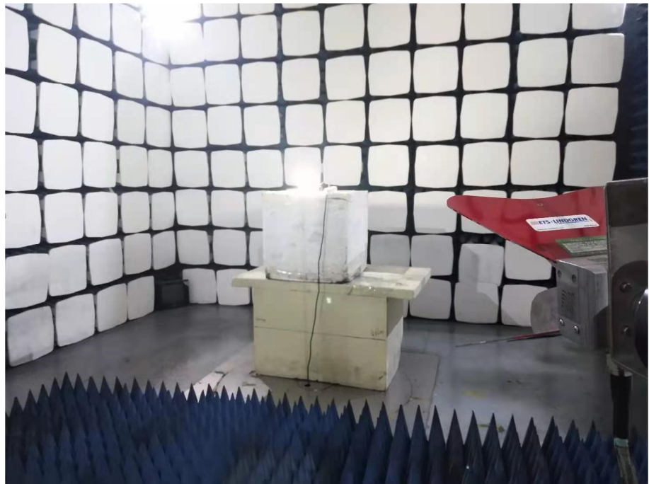
Radiation Emission Test Setup (1GHz to 18GHz)
