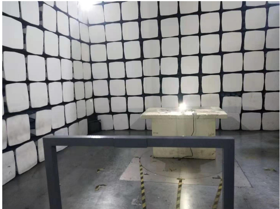
Radiation Emission Test Setup (Below 30MHz)
