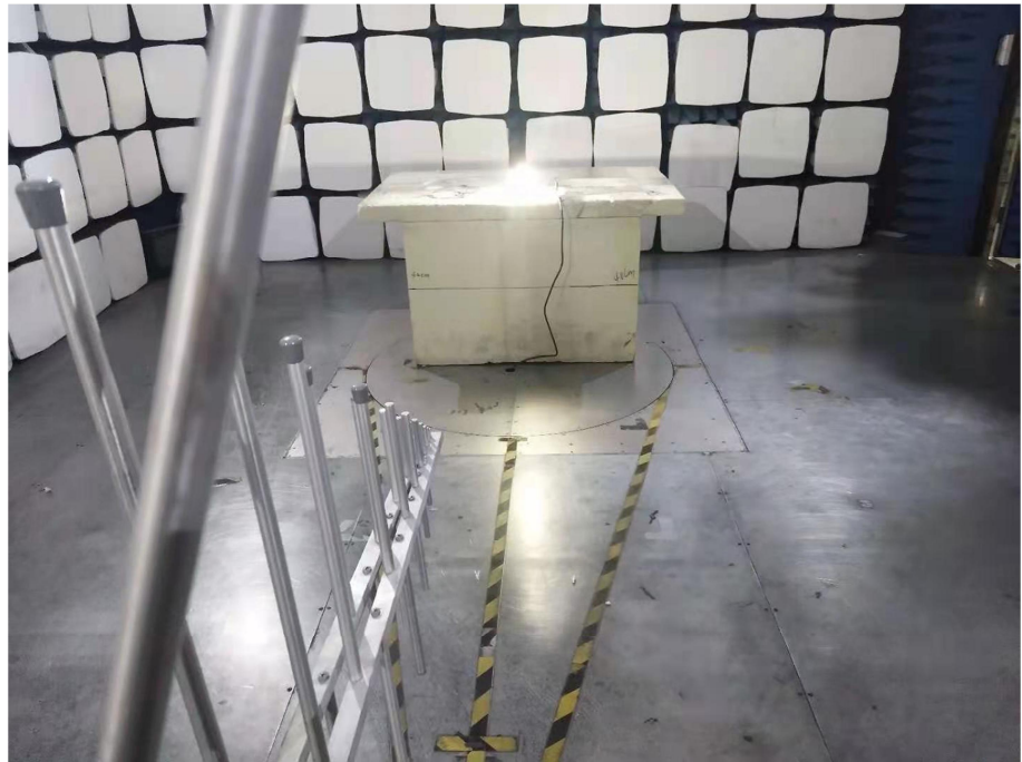
Radiation Emission Test Setup (30MHz to 1GHz)
