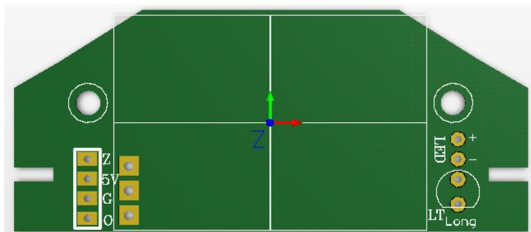
Power on,O pin after a low-level lasts for 1 minute, it becomes high-level.If the environment illumination below  $15\pm3$  Lux and there are something moving in it's detection range, then the O pin becomes low-level for 5 minutes. During this 5 minutes, if the module detects a motion, it also lasts 5 minutes else the O pin turns to high level after 5 minutes.
