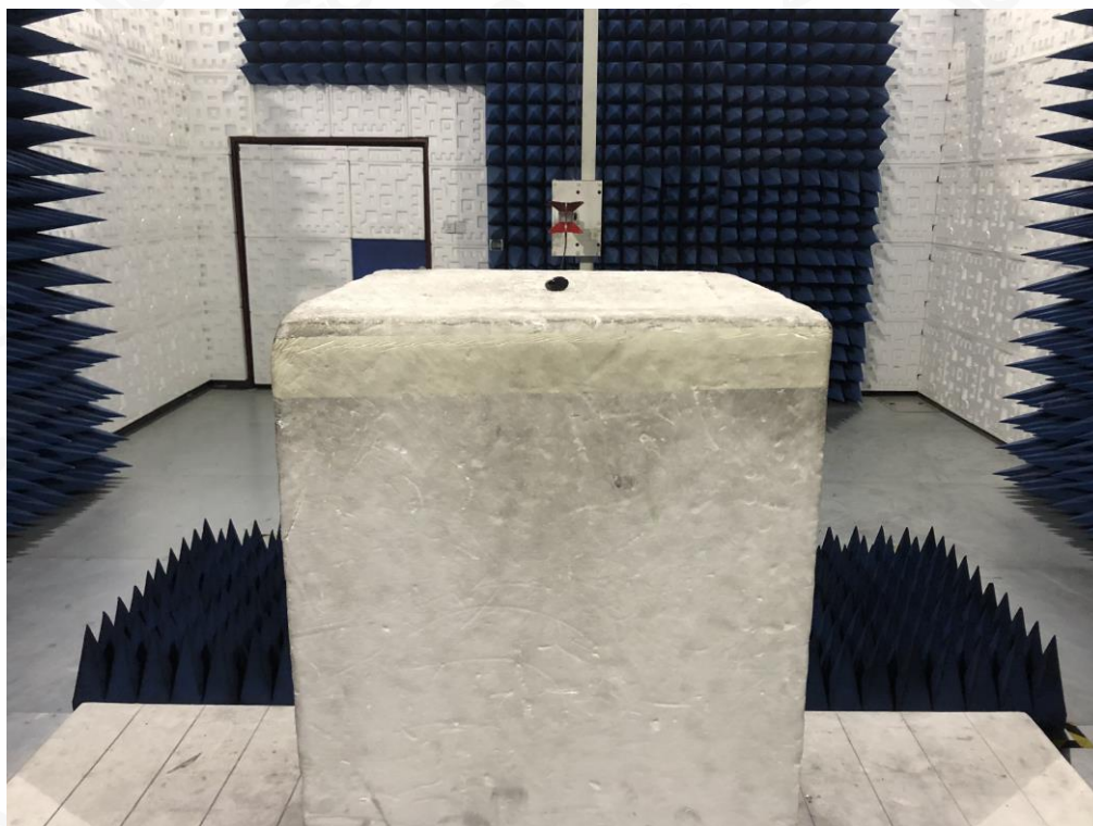
RADIATED EMISSION TEST SETUP ABOVE 1GHZ
