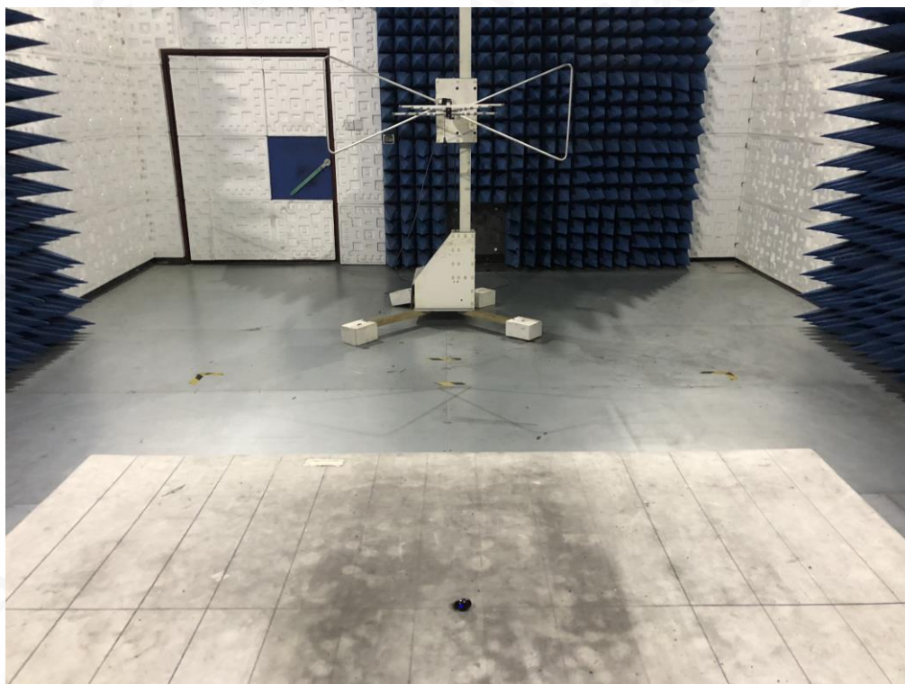
RADIATED EMISSION TEST SETUP ABOVE 1GHZ
