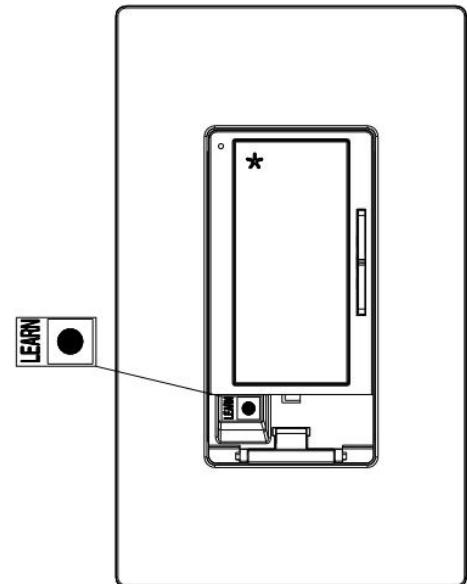
3. If user cannot finish the setting within the 60 seconds time frame, the main power must be turned off and re-started again. This will reset the unit. Repeat step 3 until the LEARNING feature is activated as indicated.
