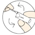
**!** To avoid breaking the Heater Blade employ a gentle circular motion when using the Cleaning Stick.
