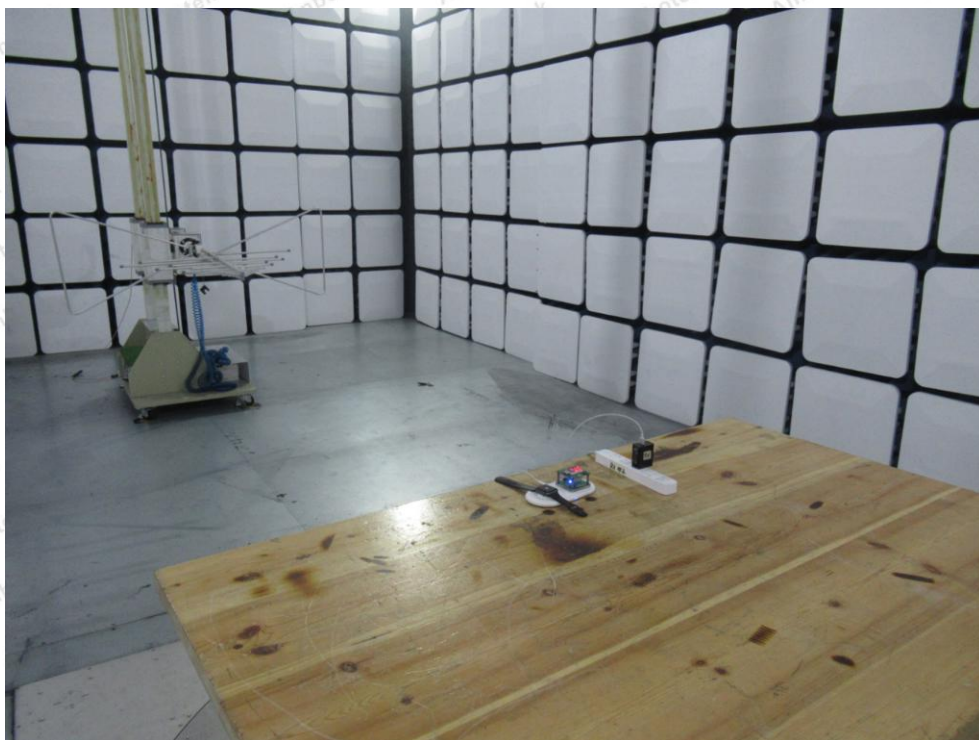
Photo of Radiation Emission Test
