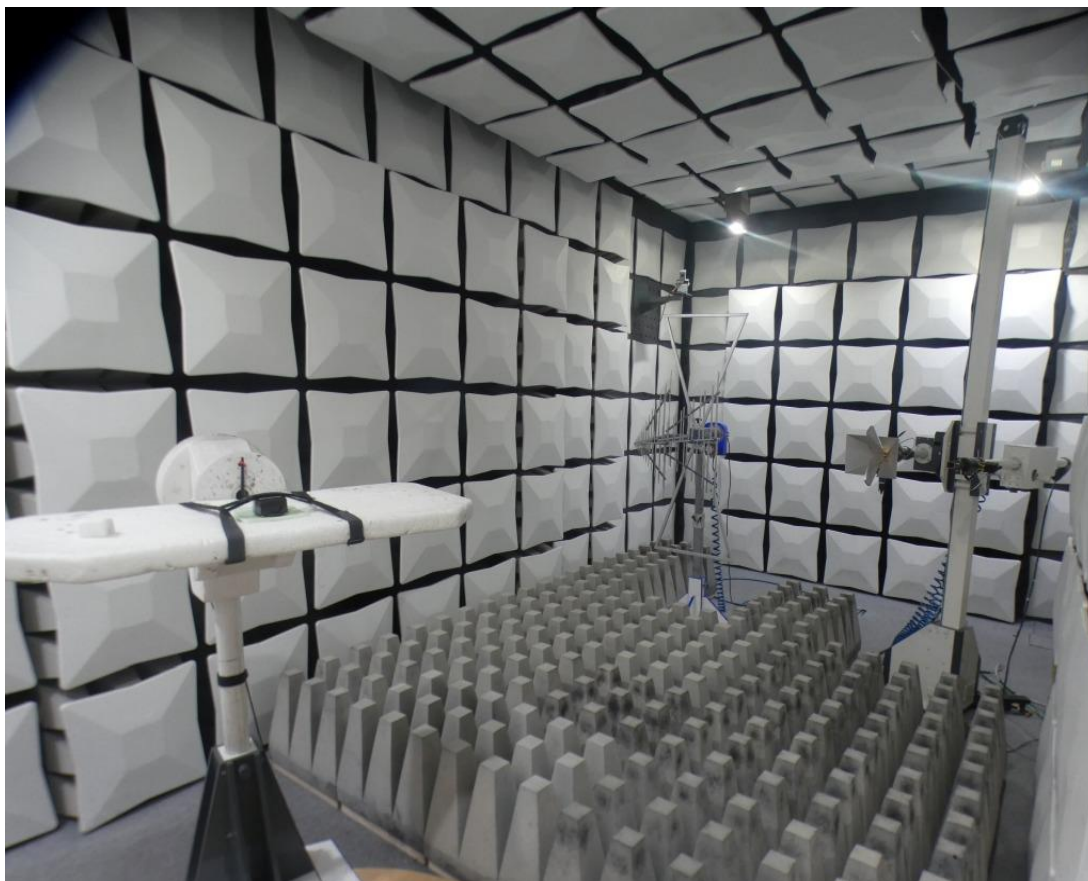
Photo 4: Test setup for radiated measurements Parts 24, 27 and FCC15.247, above 1 GHz
