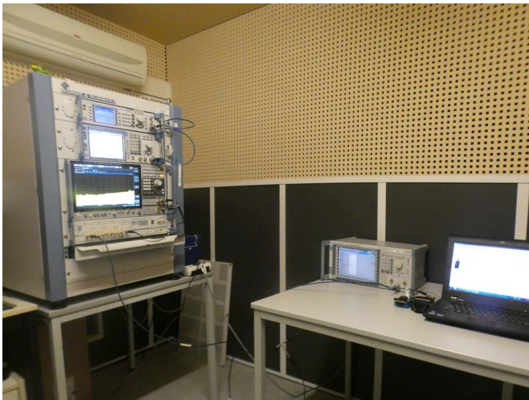
Photo 5: Test setup for conducted measurements FCC15.247
