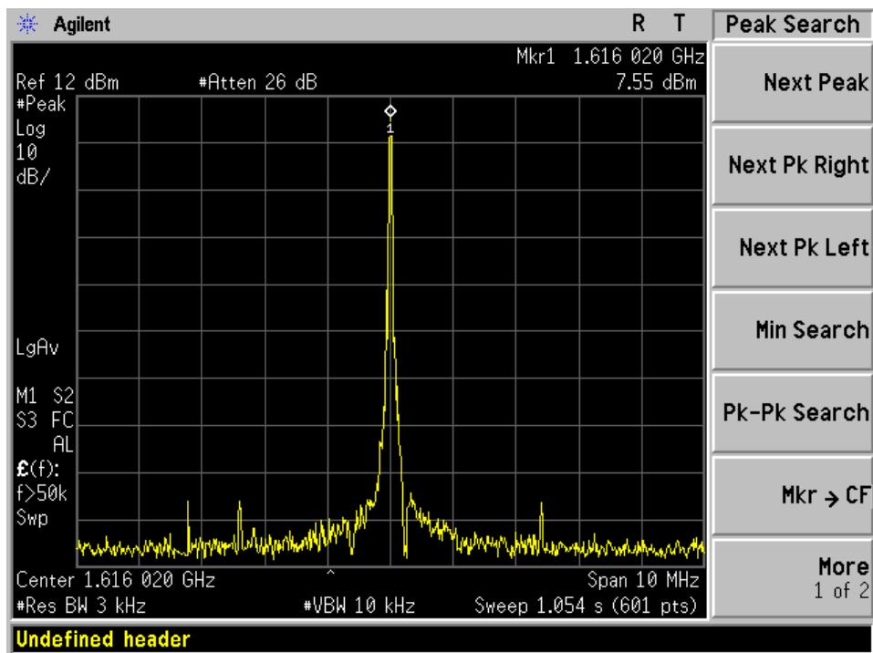
Note: Offset (dB) = 20.4dB (attenuation) + 1.8dB (cable loss) + 1.25 dB=23.45dB
