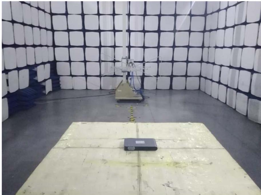
**Radiation Emission Test Setup (1GHz to 18GHz)**
