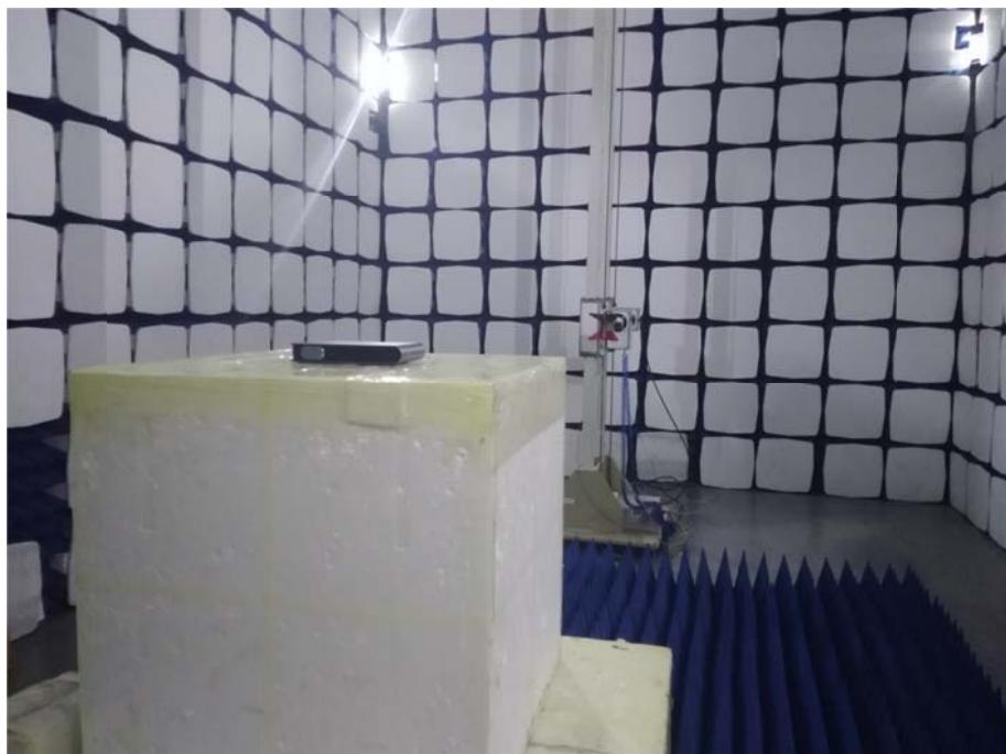
**Radiation Emission Test Setup (Above 18GHz)**
