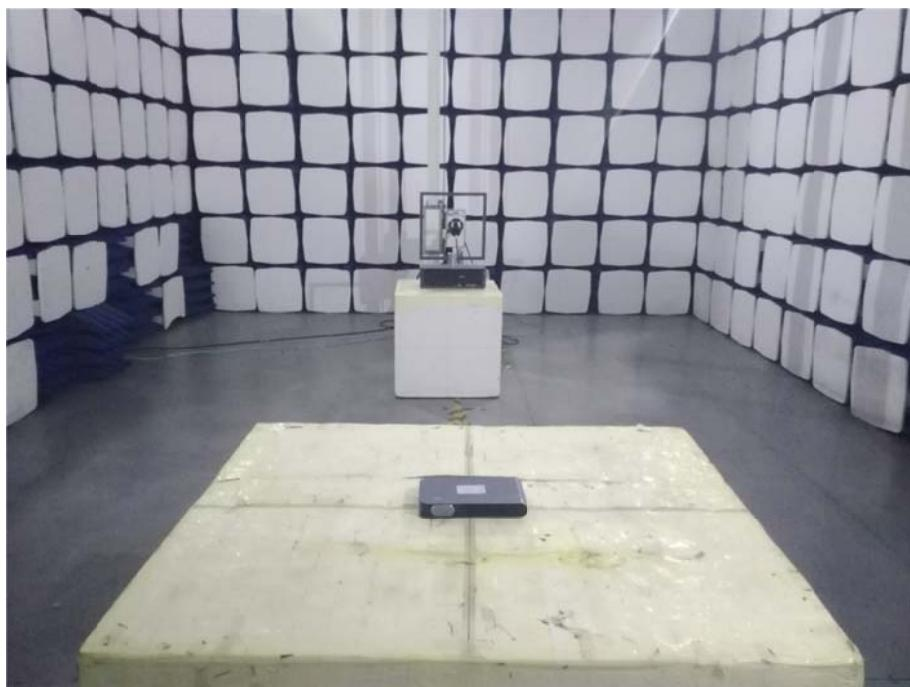
**Radiation Emission Test Setup (30MHz to 1GHz)**
