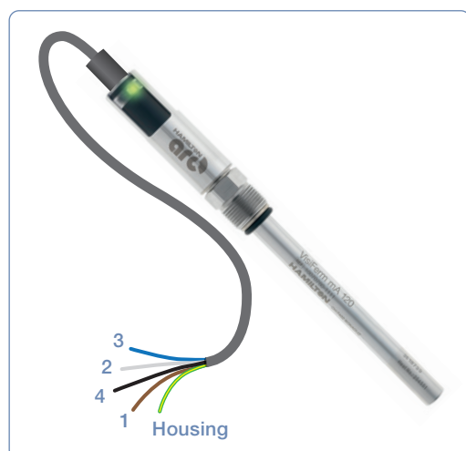
Figure 7: Requirements for electrical connection of VisiFerm mA sensors
