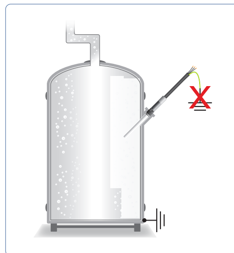
Figure 1: Metal tank with earth connection
