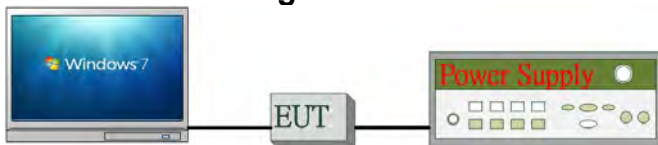
Fig. 2-2 Conducted (Antenna Port) Emission Configuration
