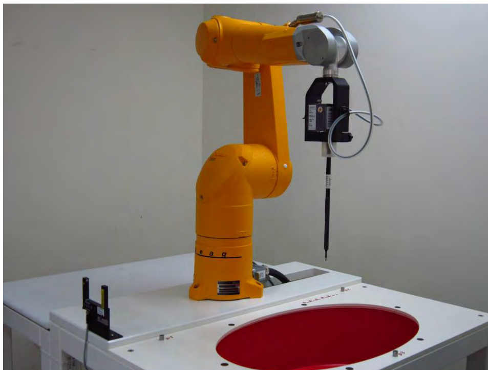
Fig.1 Photograph of the SAR measurement system
