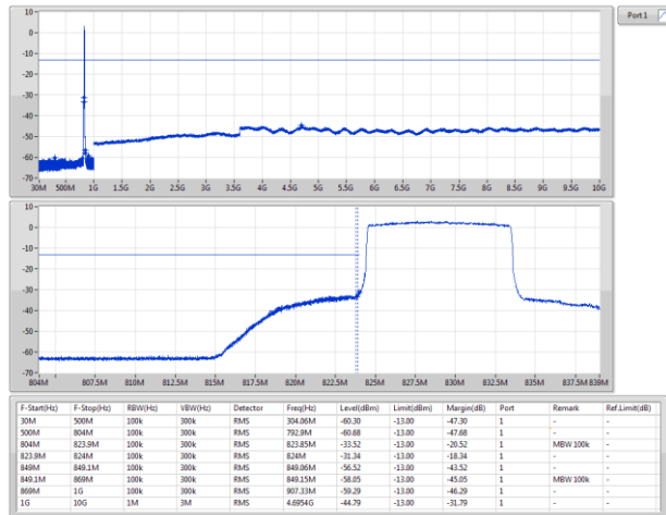
Band 5 LTE_10MHz_Nss1,16QAM_1TX 829MHz_16QAM_RB 1,#RB L
