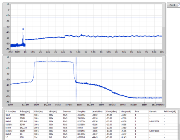
Band 5_LTE_10MHz_Nss1,16QAM_1TX 844MHz_16QAM_RB 1,#RB H
