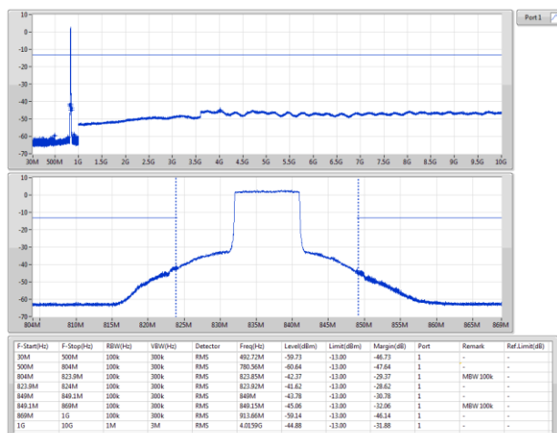
Band 5 LTE_10MHz_Nss1,16QAM_1TX 836.5MHz_16QAM_RB 50,#RB 0
